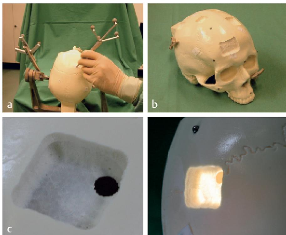
**Fig. 1** a Registration of the head using implemented markers and a navigation system, allowing constant tracking of the drill. b Results after robot milling of several craniectomies according to the analysed data of osseous tumours. c Demonstration of a layer of the tabula interna. Drilling performed by the hexapod robot.
